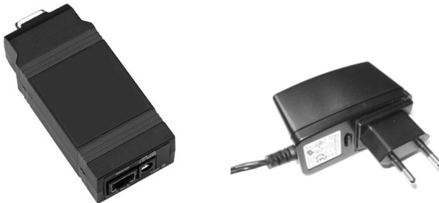
Figure 43: LMG-Z318 - external supply via wall wart
